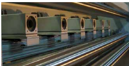
6 matrix cameras integrated in the weft straightener
