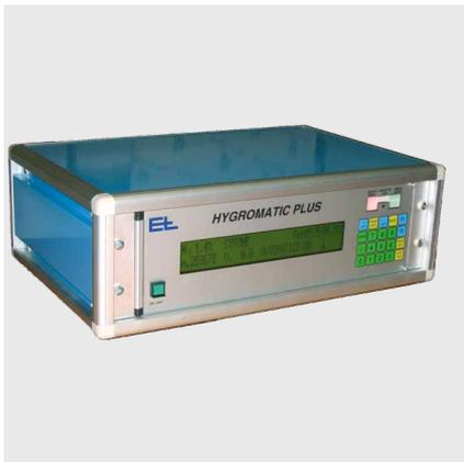
Residual moisture detector In the material
